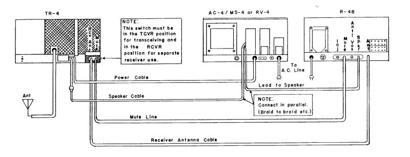
FIG. 1 USING THE R-4B WITH THE TR-4 TRANSCEIVER
